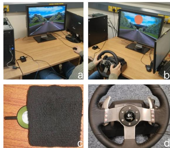
**Figure 1: The setup of Experiments 1 (a) and 2 (b), the wristband with the Tactor (c) and the steering wheel used in Experiment 2, with the response buttons (d).**
