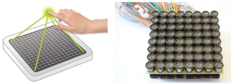
Figure 7.13 Ultrasound haptic displays use an array of ultrasound speakers, which focus sound to create a focused area of acoustic radiation pressure.
