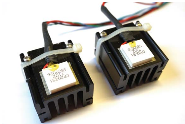
Figure 7.2 Two Peltier modules on black heat sinks, used for thermal stimulation. The white modules are placed in contact with the skin (e.g., against the palm of the hand).
