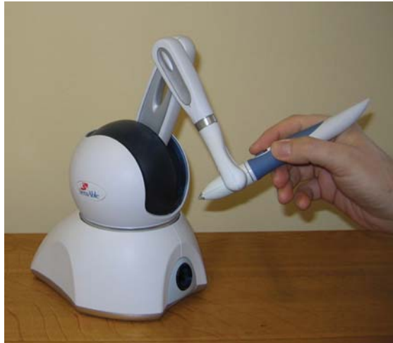
Figure 7.4 A SensAble PHANTOM Omni (now Geomagic Touch) with pen attachment. (From McGookin and Brewster [2006])
