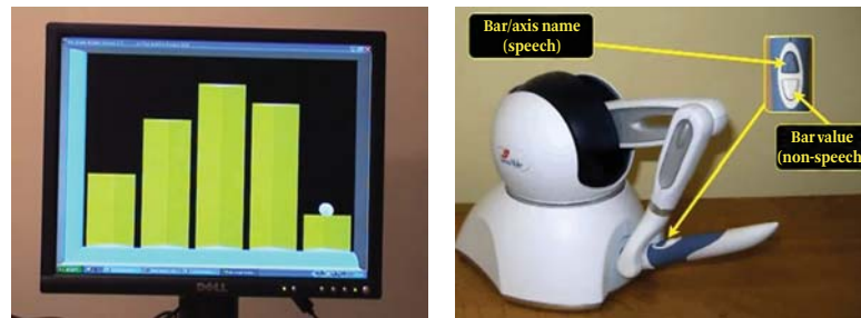
Figure 7.7 Left: Screenshot from a video demonstration of McGookin and Brewster [2006] auditory system for navigating data sets. Link to video: http://bit.ly/2nFZ6sD . Right: Screenshot from a further video demonstration of their work. Link to video: http://bit.ly/2mKtvaa . These videos show the combined use of force feedback and sonification of tabular data.
